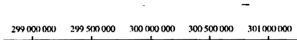
Figure 5.4 The velocity of light is given as 300\,000\,000 to three significant figures. It must therefore lie in the range 299\,500\,000 to 300\,500\,000
